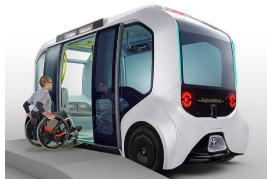
Figure 6: Toyota's e-Palette, an electric AV designed to accommodate up to four wheelchair-bound passengers with additional riders; Source: Toyota
