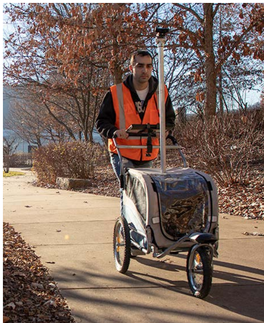
Figure 18: The pathMet device is a sidewalk profiling tool that measures compliance with ADA guidelines to provide accessible wayfinding for all; Source: pathVu
