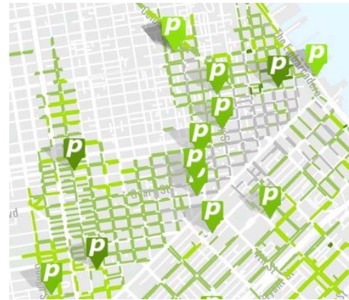
Figure 3: A screenshot from San Francisco’s smart parking initiative. The street parking and city-owned garages with demand-based pricing are shown in green gradient, with darker green being more expensive per hour; Source: SFMTA
