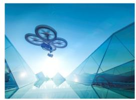
The UAS data collection includes lidar, GPS, video, and photogrammetry. The combined dataset is processed into a 3D mesh model with photo overlay and used by inspectors to perform virtual inspections. Th 3D digital twin of the structural asset can also be included in other immersive/XR technology to conduct safe, efficient training.
